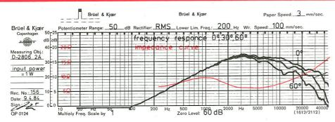
The 30° and 60° off-axis curves prove clearly that the special house construction has no directional/horn effect at all.
