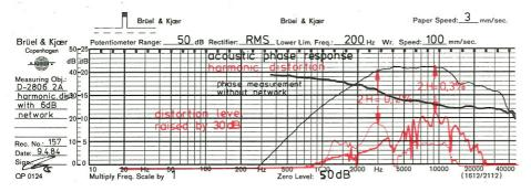
The acoustic phase runs linear up to 50 kHz.
