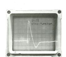
The rise time of a speaker is measured by means of a STEP-FUNCTION. The total is set to be 100 %, then 10 % and 90 % are marked. The first 10 % is the phase of acceleration, the last 10 % is the deceleration phase of the diaphragm. The 80 % between both marks are defined as the movement of the diaphragm. The time needed for this phase is called the rise time. The step function of the D-28 often is used as a scientific example because of its linearity.
