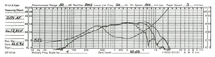
Frequency response and impedance curve of the D-54 AF, distance: 1 m, on-axis, 30° and 60°.
